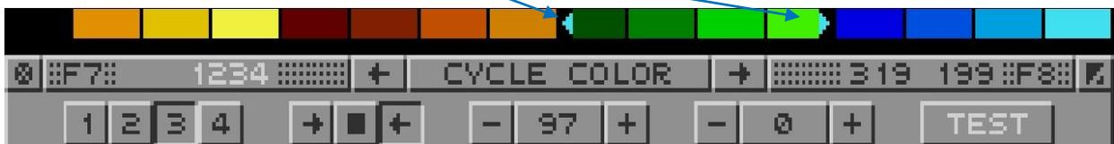
**1 to 4 ② Color Cycles** *Selecting a cycle, sets the cycle direction and limiting sliders on the palette*
