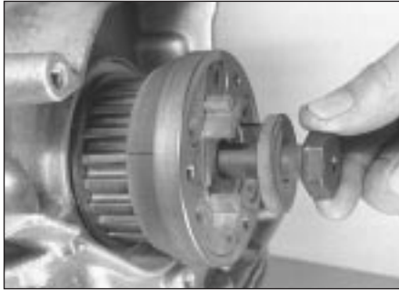
12.34a Removing crankshaft sprocket bolt . . .
