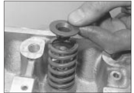
13.3a ... and remove spring cup retainer, spring ...
