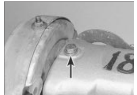
22.9 Copper washer (arrowed) under bolt head
