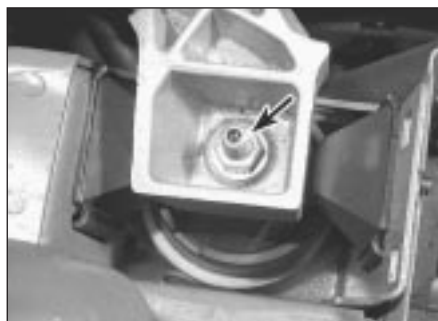
8.31 Right-hand engine mounting through-bolt (arrowed)
