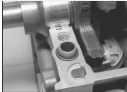
17.20 Crankcase flange O-ring seal in position on dowel
