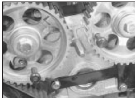
5.12a Camshaft sprocket locking pins in position
