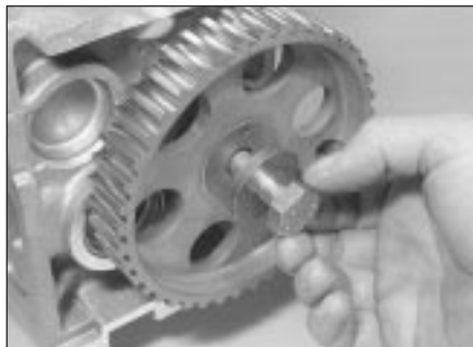
14.1b Unscrew camshaft sprocket bolt ...
