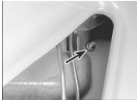
17.8 Door outer handle retaining nut (arrowed)
