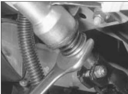
16.10a Use a spanner to compress the spring and washer . . .
