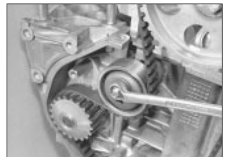
6.8 Loosening timing belt tensioner roller nut
