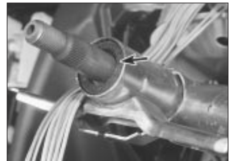
16.17 Upper steering column oil seal (arrowed)
