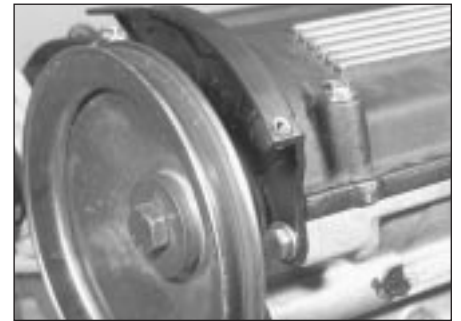
16.36 Camshaft plastic guard and pulley correctly refitted
