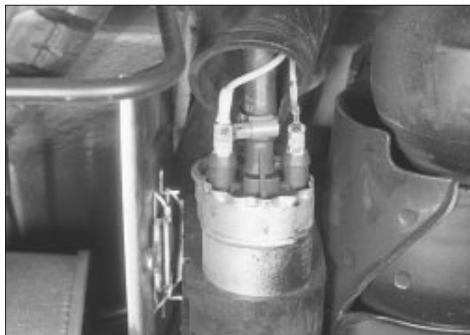
4.5 Fuel pump wiring connections
