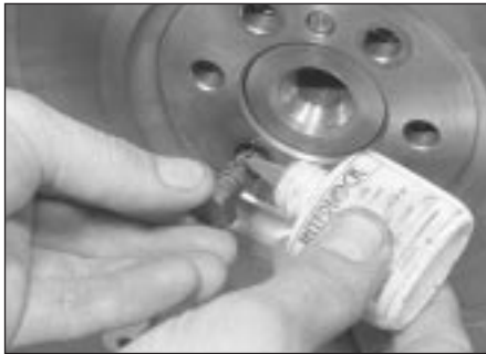
18.25 Applying locking fluid to a flywheel bolt
