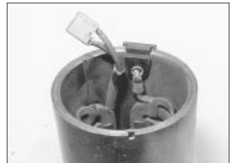
10.7 Brush connections to field coil
