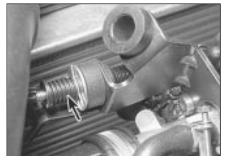
13.1 Accelerator cable adjustment ferrule (arrowed)
