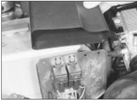
2.6 Fuel injection system relays (BX 19 GTi with Bosch LE3 Jetronic fuel injection)
