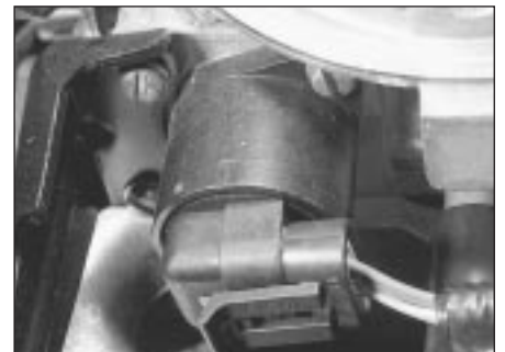
15.1 Idle control stepper motor location
