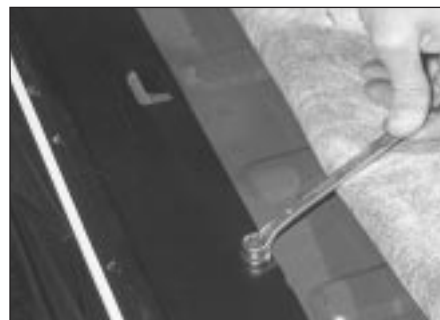
26.4 Unscrewing rear seat back hinge bolt
