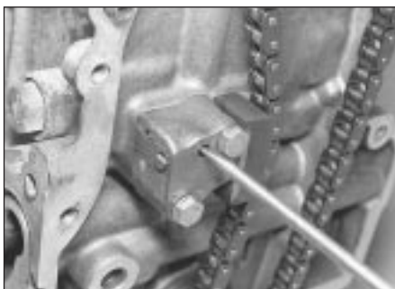
17.36 Releasing timing chain tensioner - first type
