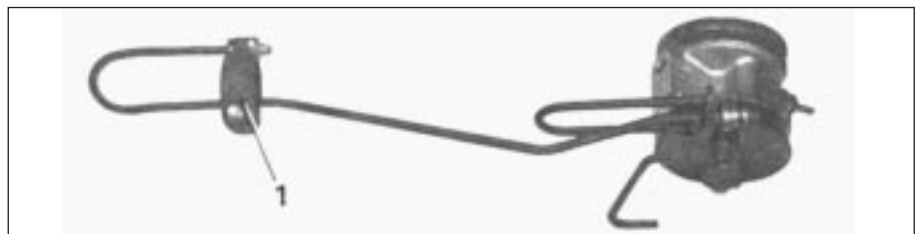
12.5a Front height corrector adjustment - move collar (1) as required around anti-roll bar
