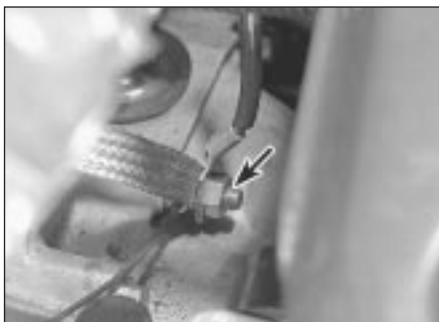
8.27 Earth cables at transmission (arrowed)
