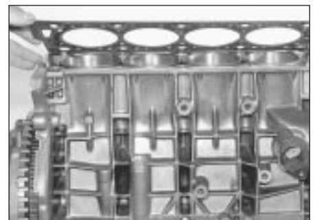
6.28 Fitting a new cylinder head gasket
