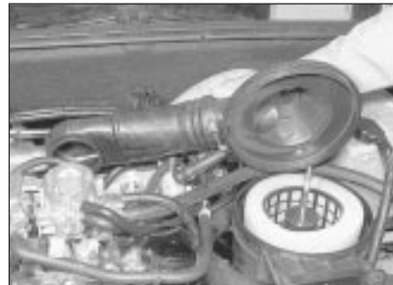
28.7 Lift off the cover, complete with inlet duct to expose the air filter element - BX 16 and BX 19
