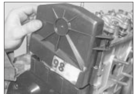
6.5b Removing upper timing cover
