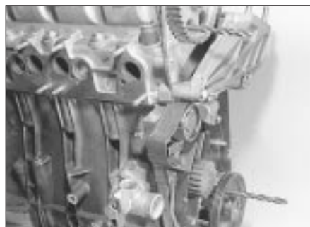
6.4b Timing dowels (drills) in position
