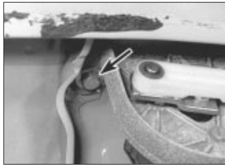
19.6a Wiper motor retaining bolt (arrowed)
