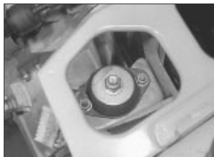
9.31 Left-hand side transmission mounting
