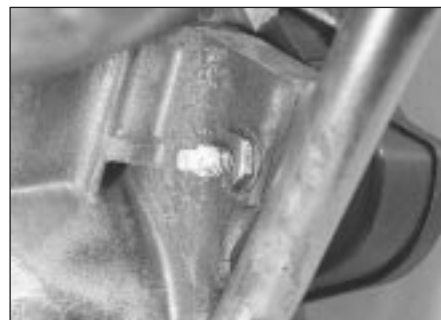
6.8 Tensioner cam spindle (square end) and locknut
