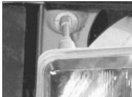
3.6 Headlamp ball and socket mounting
