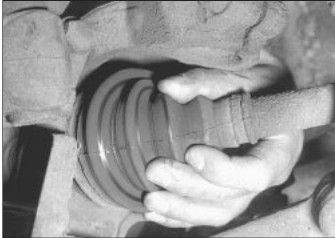
17.1 Inspect the CV joint rubber bellows for signs of cracking, splits or deterioration
