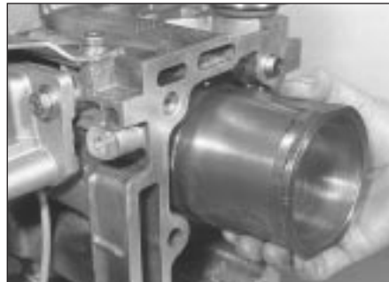
12.45 Removing a liner/piston assembly
