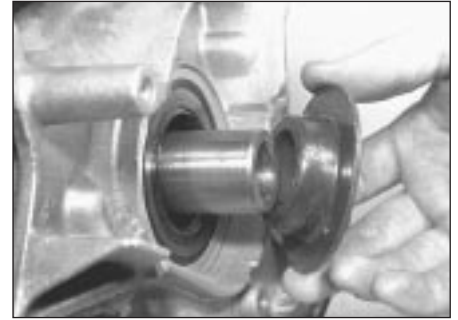
12.34c . . . and timing belt guide plate
