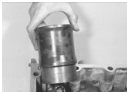
17.12 Installing piston/liner assembly
