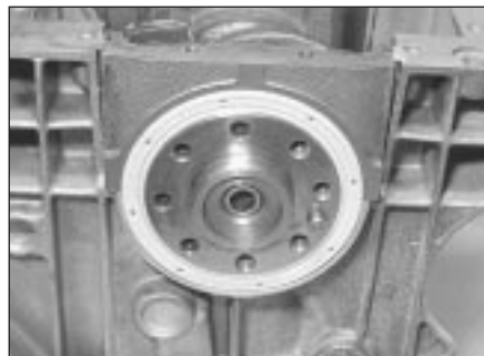
19.15 Crankshaft oil seal - flywheel end
