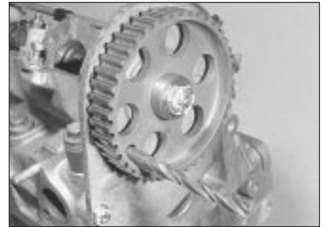
13.12 Lock camshaft sprocket with a 10 mm rod
