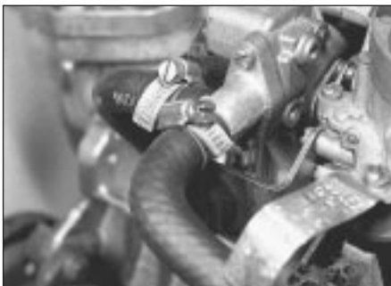
14.8 Solex 32-34 - coolant hose connections
