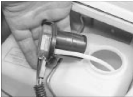
22.2 Washer unit filler cap/pump unit
