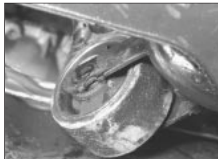
8.16 Engine rear mounting and yoke
