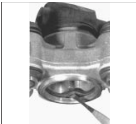
4.15 Prise free the cylinder inner seal
