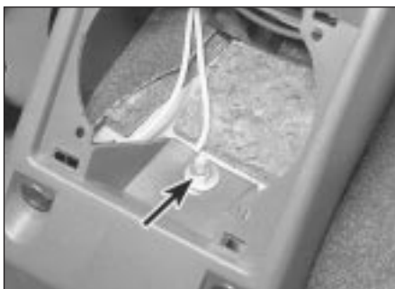
13.2 Handbrake console retaining nut (arrowed)
