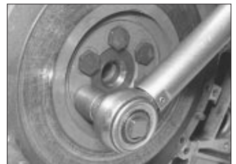
18.14 Tightening flywheel bolts to specified torque
