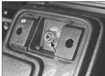
16.15b . . . to expose wheel retaining nut (arrowed)
