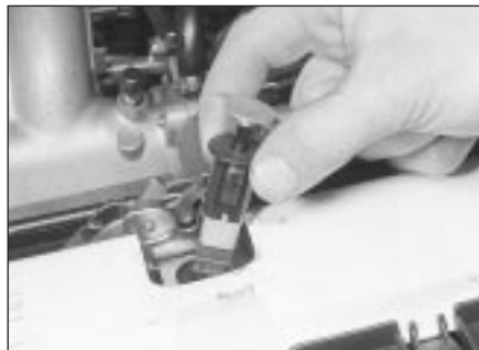
26.4 Removing the bonnet-open warning switch
