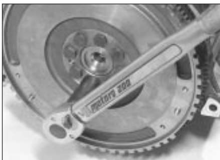
16.20 Tightening a flywheel bolt
