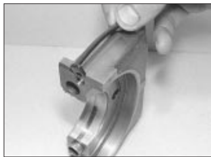
19.10a Fitting a side seal to No 1 main bearing
