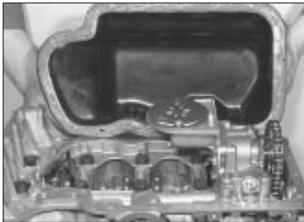
12.39 Removing the sump
