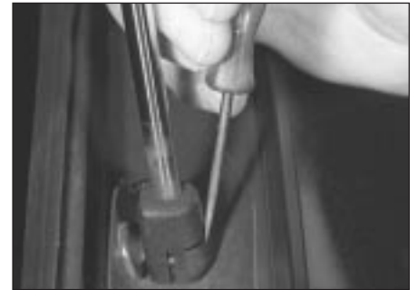
19.11 Prising out tailgate strut balljoint clip
