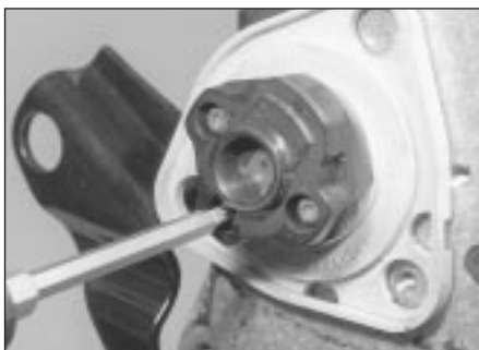
7.3 Removing a rotor arm securing screw - GTi 16v with Motronic ML4.1
