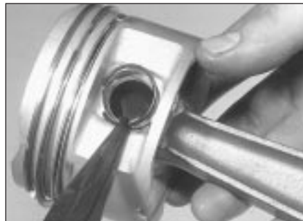
16.9b Inserting a gudgeon pin circlip
