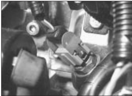
11.13 Fuel/air mixture temperature sensor location
