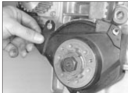
6.5d Removing lower timing cover
