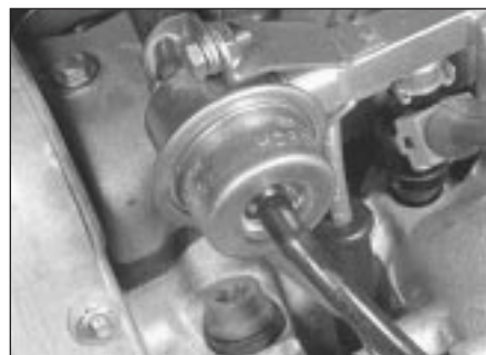
12.4b Pressure regulator attached to fuel rail
