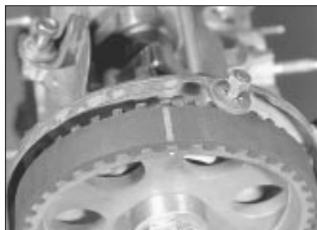
6.10b Line on belt aligns with mark on camshaft sprocket
