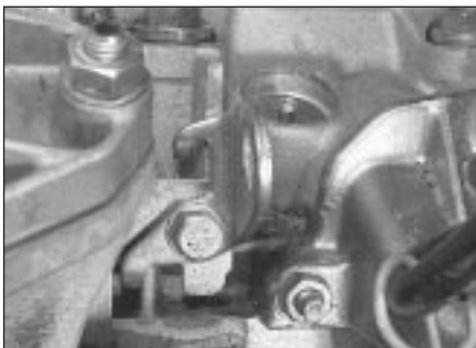
9.29 Engine lift support bracket - front right-hand side
