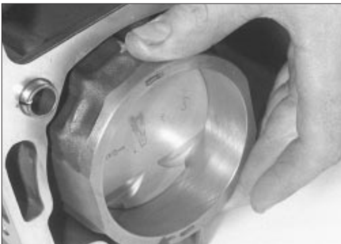
16.12a Fitting a piston/connecting rod/liner assembly
