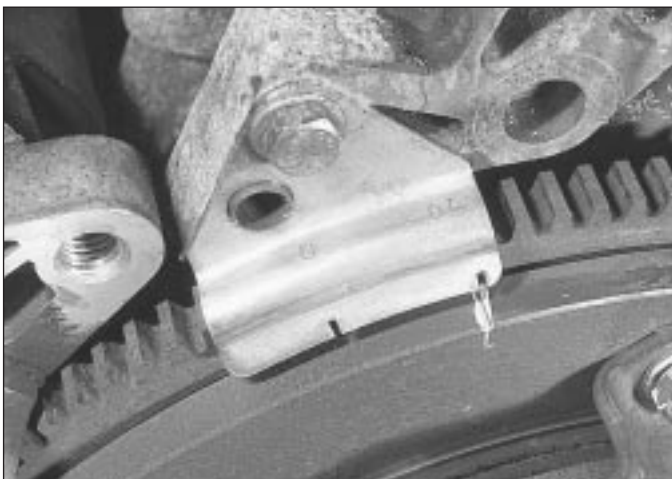
8.2 Flywheel timing mark aligned with advance timing mark on timing plate - BX 16
