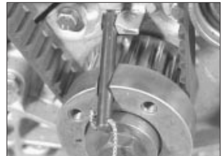
5.12b Crankshaft sprocket locking rod in position
