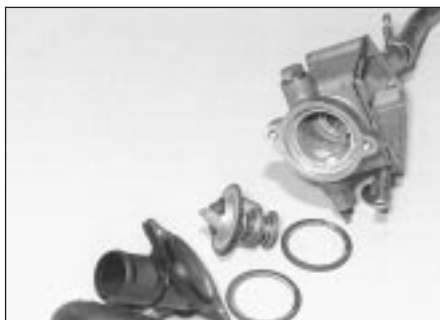
8.1b Thermostat housing dismantled - BX 19 GTi 16v
