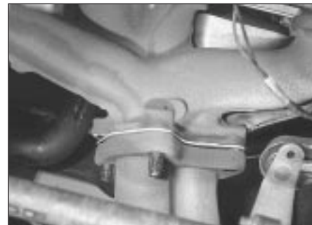
25.3b Exhaust manifold-to-downpipe connection - BX 16
