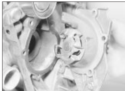
10.12 Coolant pump removal
