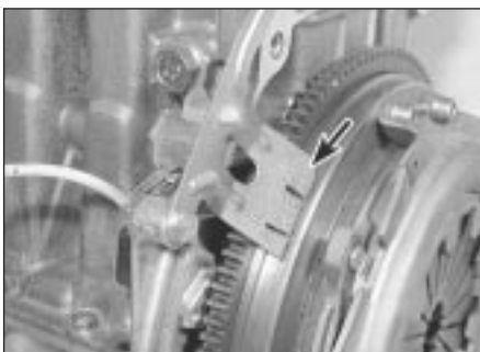
7.20 Timing plate (arrowed)
