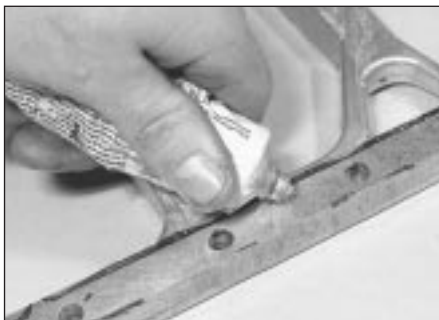
16.18 Applying instant gasket to sump spacer plate
