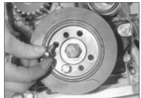
5.18b Fitting a crankshaft damper bolt
