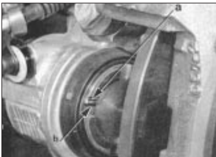
2.10 Piston alignment position with identification mark (a) above (or below) piston groove (b)
