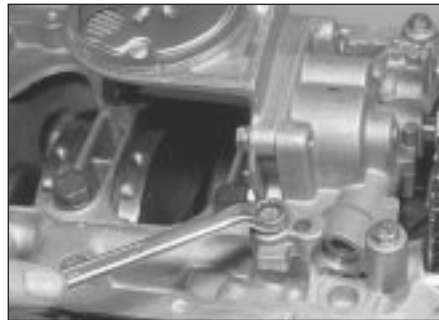
12.40a Unscrew oil pump retaining bolts . . .
