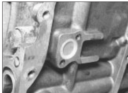
17.29a Locate chain tensioner filter . . .
