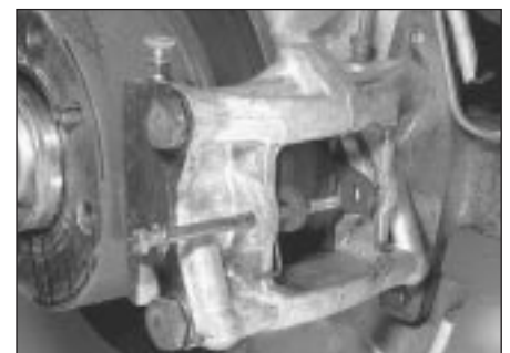
2.25 Locating the through-bolt
