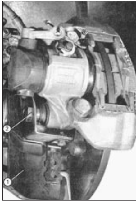
4.8 Front brake caliper deflector (1) and retaining bolt (2)
