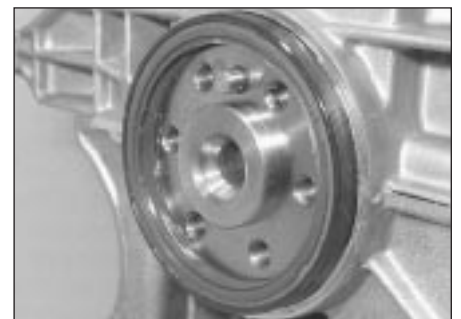
18.23 Crankshaft rear oil seal located over rear of crankshaft
