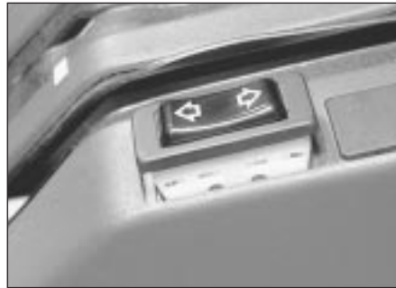
11.2 Electric window operating switch removal
