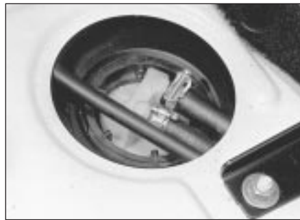
7.2 Fuel tank supply and return hoses - GTi
