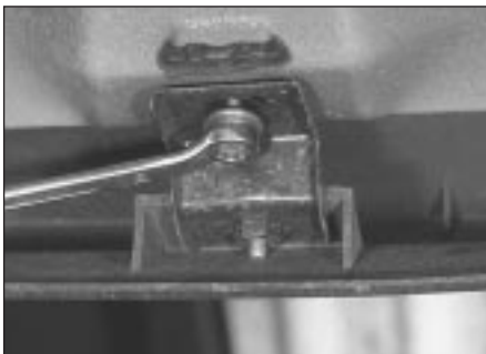
20.11a Unscrewing a rear bumper lower screw
