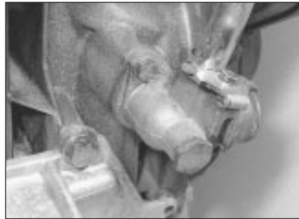
19.49a Securing coolant pipe to inlet housing
