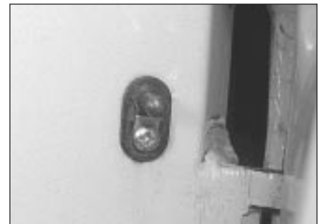
10.2 Door courtesy light switch retaining screw
