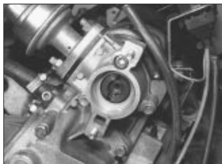
6.9 Distributor drive engagement dog is offset - BX 16
