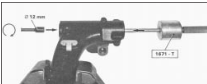
8.12 Rear suspension arm bearing removal tools
