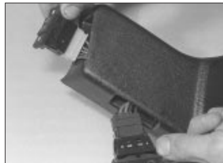
12.9b Window regulator switches withdrawn to expose wiring
