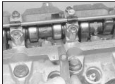
22.5b Measuring a valve clearance - 171 and 159 engines
