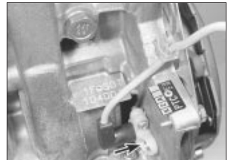
7.19 TDC sensor mounting bolt (arrowed)
