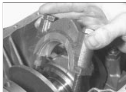
16.5b Fitting a main bearing cap
