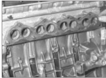
6.38a Exhaust manifold gasket correctly located
