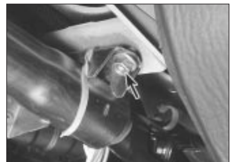
19.4 Steering column upper retaining nut (arrowed)
