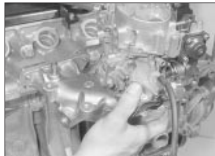
7.9 Removing inlet manifold complete with carburettor
