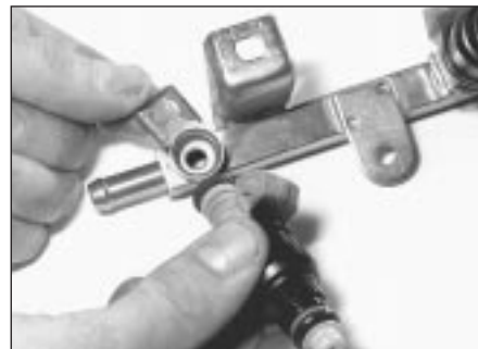
11.1 Removing a fuel injector from the rail
