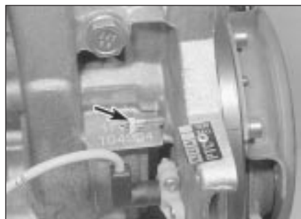
6.7 Using long bolt (arrowed) to align TDC holes in flywheel and cylinder block
