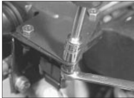
11.18a Slacken and remove the three retaining nuts and bolts . . .
