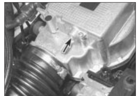
9.3 Mixture adjustment screw (arrowed)
