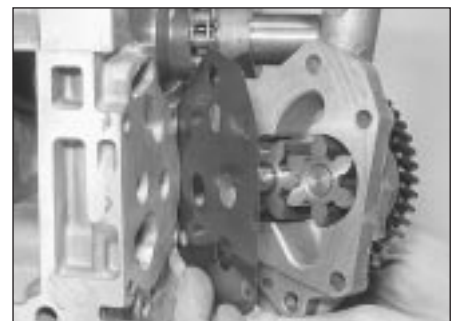
17.39 Fitting oil pump with spacer plate
