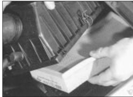
28.18a . . . remove the lid and withdraw the air filter element - Magneti Marelli system
