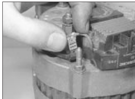
7.4a Disconnect the regulator lead . . .
