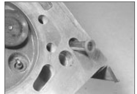
15.12 Insert oil filter gauze in cylinder head oilway
