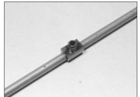
14.15 Pinholes of lubrication manifold must be clear
