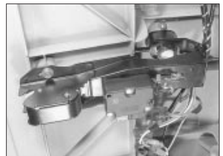
25.10 Tailgate central locking solenoid and lock unit
