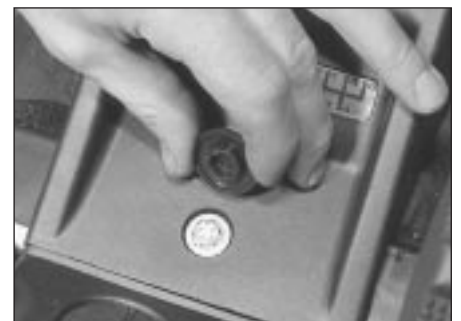
25.1 Removing plastic cover for access to centre console retaining bolt
