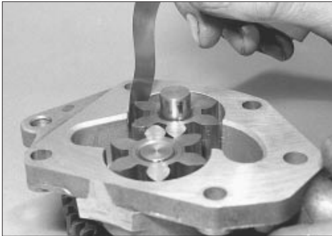
12.41 Checking oil pump lobe tip clearance
