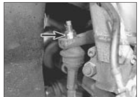
3.11 Anti-roll bar and connecting rod. Remove retaining nut (arrowed)
