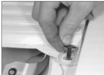
13.14 Removing an air inlet grille securing clip
