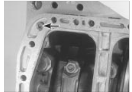
11.32a Extract Allen screws (arrowed) . . .
