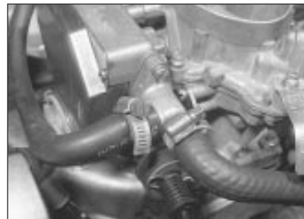
8.5b Coolant hose connections to carburettor auto-choke
