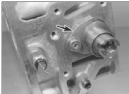
14.2 Camshaft thrust fork (arrowed)
