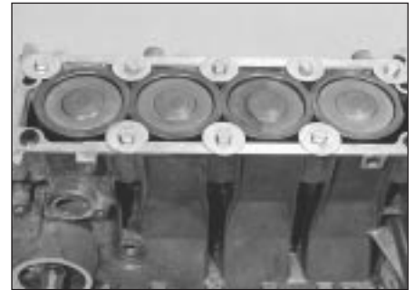
16.4 One method of clamping cylinder liners
