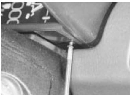
7.12 Unscrewing a trim panel retaining screw
