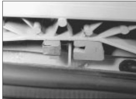
19.7 Tailgate hinge retaining clip
