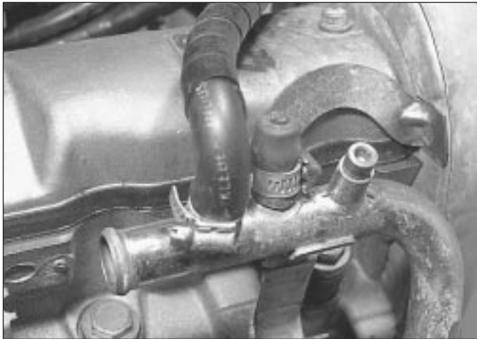
8.6a Heater coolant hose and support clamp
