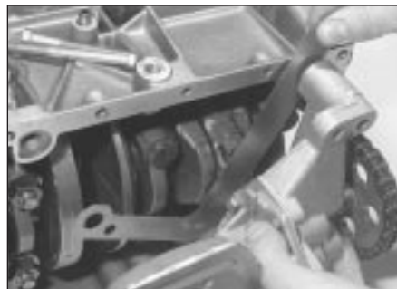
11.34c Removing oil pump drivechain tension adjustment shim
