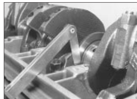
17.17 Checking crankshaft endfloat
