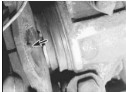
3.0b Locating pip (arrowed) on onboard pad
