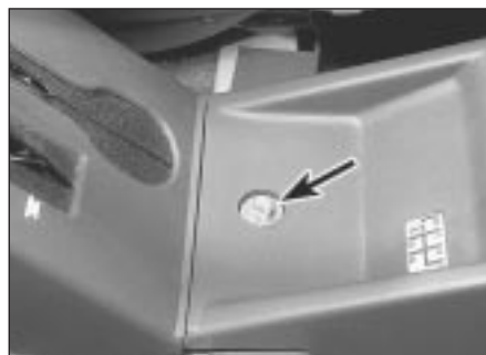
13.3 Console retaining bolt (arrowed)
