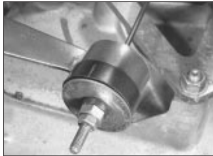
8.24 Clutch cable connection at release lever
