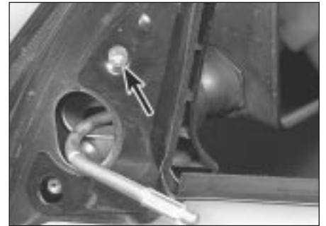
10.3 Countersunk screw retaining the inner plate (arrowed)
