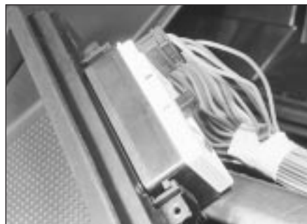
15.4 Clock unit rear detail - unclip to remove
