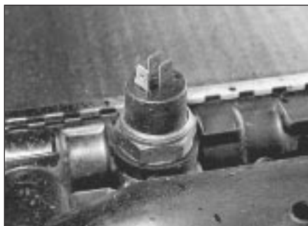
3.3 Temperature sensor unit location in radiator
