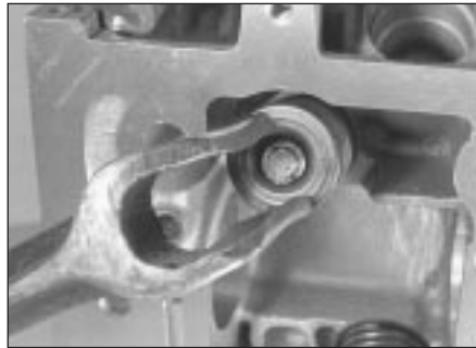
14.4a Compress valve spring and remove split collets ...
