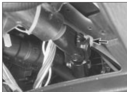
19.3 Steering intermediate shaft universal joint (arrowed)
