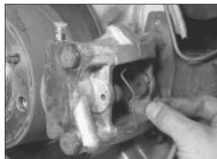
2.19a ... withdraw spring retainer clip ...
