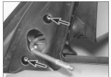
10.4 Door mirror retaining nuts (arrowed)
