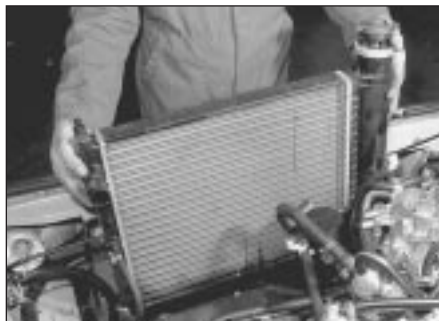
3.5 Lifting radiator out of vehicle
