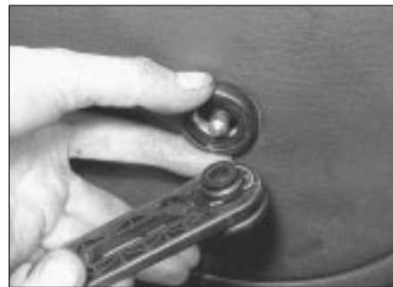
12.1 Removing the window winder handle (manual type)
