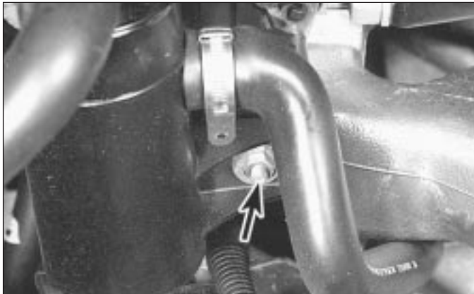
16.4 Oil filler/breather cap retaining nut (arrowed)
