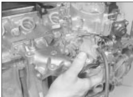
6.14 Timing cover correctly refitted
