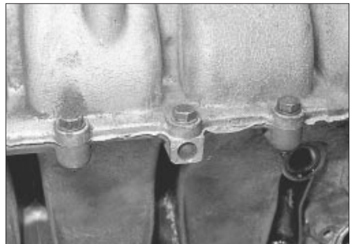
17.26 Crankcase housing flange bolts
