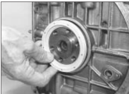
17.27 Fitting new crankshaft oil seal
