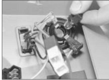
4.4c Removing the map reading light bulb
