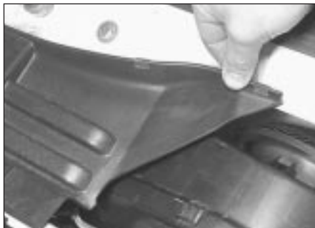
13.13 Removing plastic cover from heater blower motor
