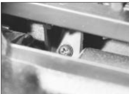
7.15 Instrument panel lower retaining screw
