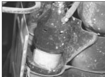
5.1 Fuel pump location - GTi 16v with Motronic ML4.1
