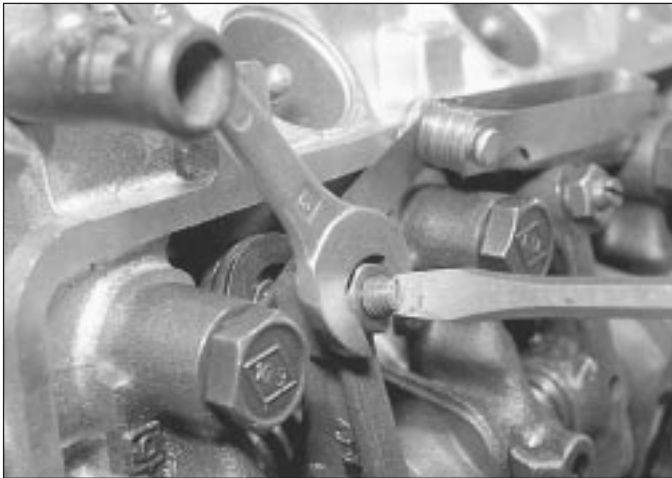
21.6 Adjusting a valve clearance - 150 engine
