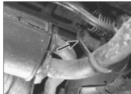
26.3 Exhaust system flexible hanger (arrowed)
