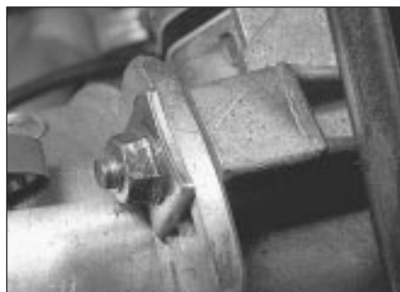
6.6 Distributor timing alignment mark - BX 16
