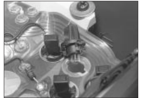
7.7 Bulb holder removal from the instrument panel
