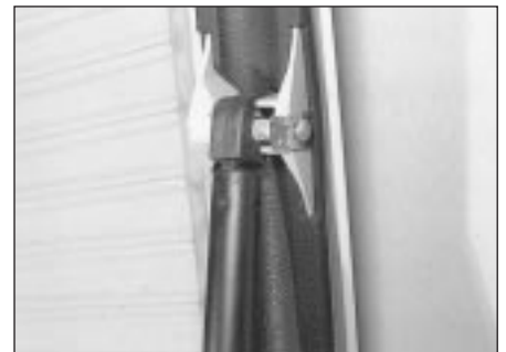
19.6a Support strut and retaining clip to tailgate
