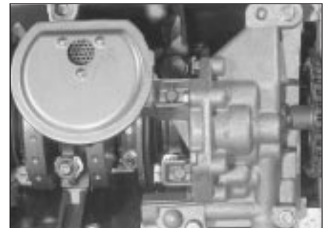
11.34a Oil pump in position
