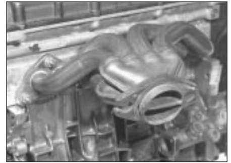
6.38b Exhaust manifold fitted
