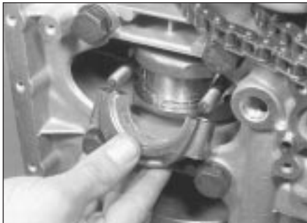
12.44 Removing a big-end bearing cap
