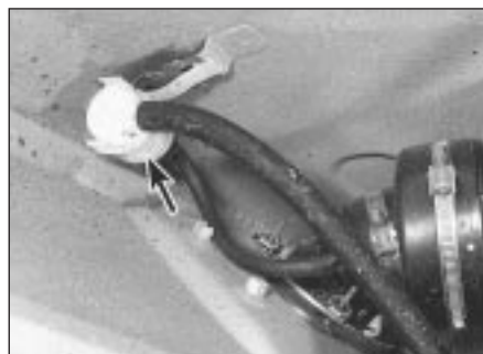
8.3 Vent valve location (arrowed) - GTi
