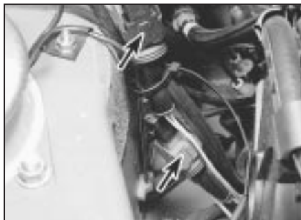
11.5 Lambda sensor wiring connectors (arrowed) situated in right-hand corner of engine compartment
