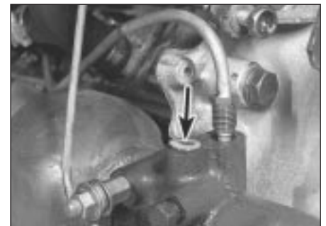
4.4 Disconnecting the rigid pipes from the pressure regulator. Note the plug inserted into the vacated port (arrowed)
