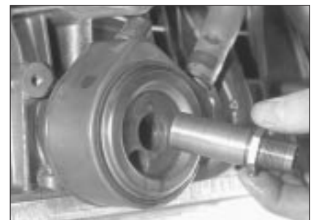
16.32 Fitting oil cooler retaining tube and nut
