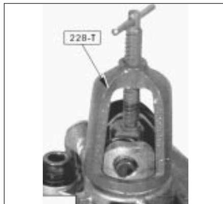
4.20a Using special tool to compress the dished spring washers
