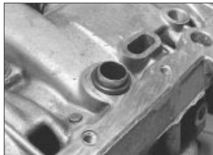
18.6 O-ring seal on transmission casing
