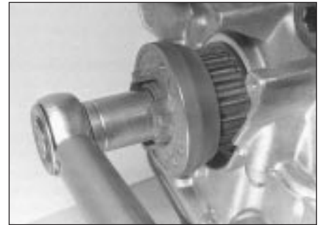
18.28 Tightening crankshaft sprocket bolt
