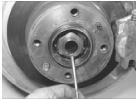
7.13 Stake lock the new hub nut to secure it
