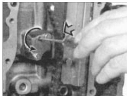
11.3a Loosening first type chain tensioner
