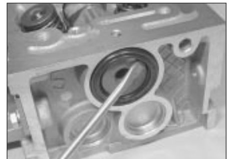
14.3a Prise out camshaft oil seal ...
