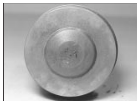
17.6 Piston crown showing directional arrow
