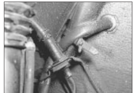
4.4 Rigid brake line connection under front wheel arch
