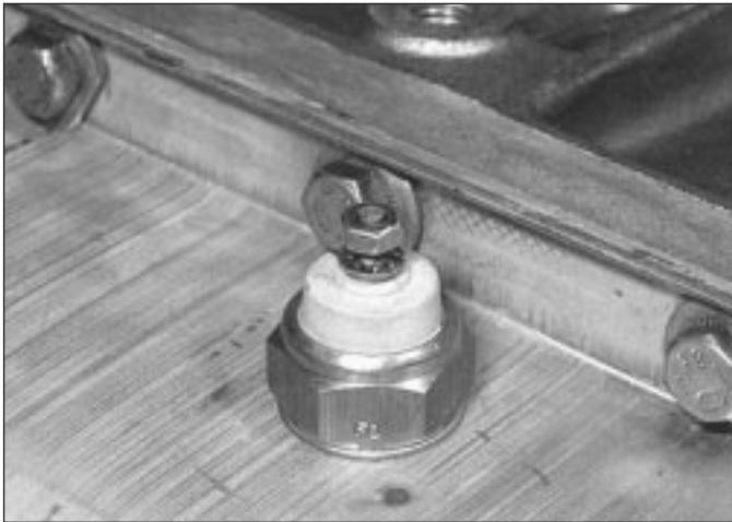
16.34 Oil temperature switch in sump pan
