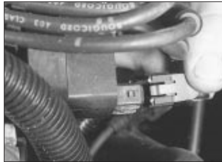
5.8 Disconnect ignition coil wiring connector
