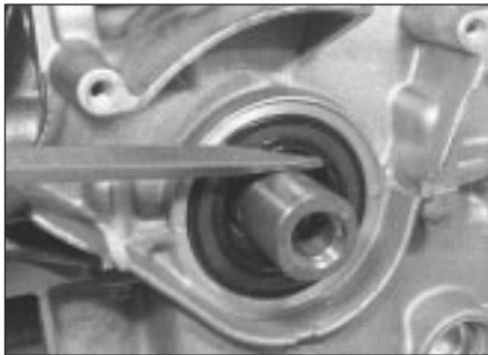
12.35 Prising out crankshaft front oil seal
