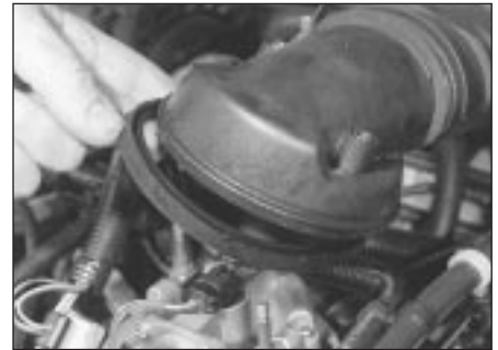
12.1b . . . then disconnect inlet trunking and remove rubber sealing ring
