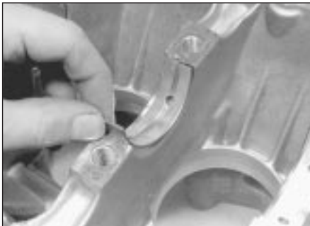
12.51a Removing a main bearing shell ...
