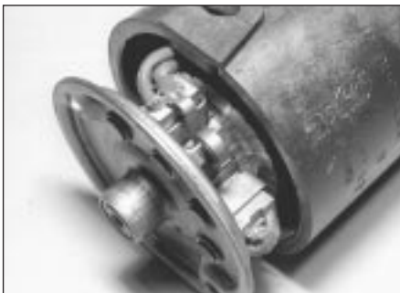
10.4 Removing bearing plate
