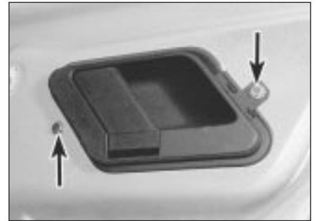
17.10 Door inner handle and retaining bolts (arrowed)
