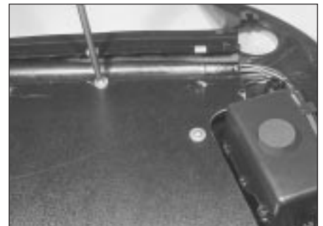
12.10 Extracting a screw from the window regulator mounting panel
