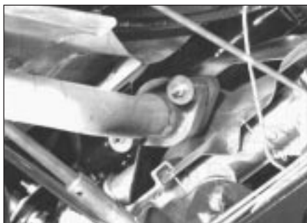
6.7 Exhaust downpipe ball socket connection
