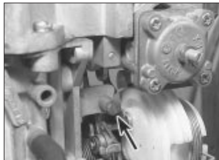
23.6c Idle speed adjustment screw (arrowed) - Solex 32-34 carburettor
