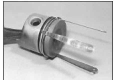
17.1 Method of fitting piston rings
