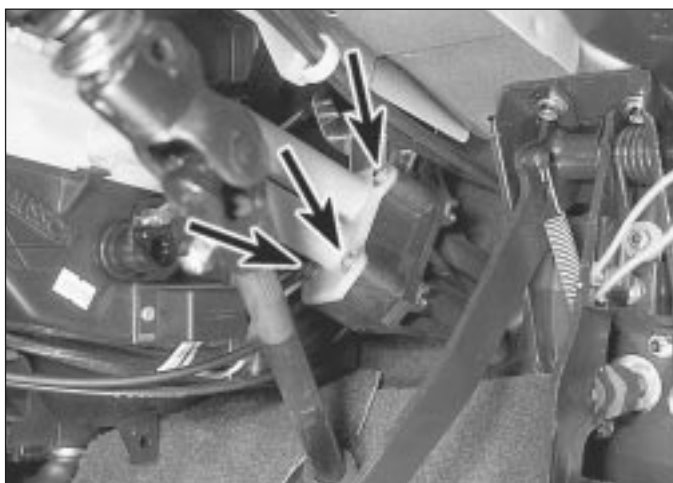
14.3 Heater tap (control) unit retaining screws (arrowed)
