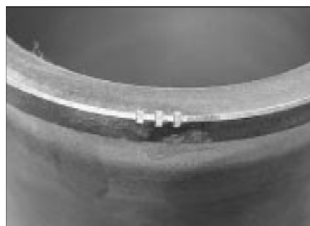
17.4 Piston/liner grading mark
