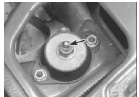
8.30a Left-hand engine mounting through-bolt (arrowed)
