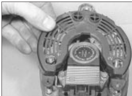
7.3 Removing the rear shield - Paris-Rhone alternator
