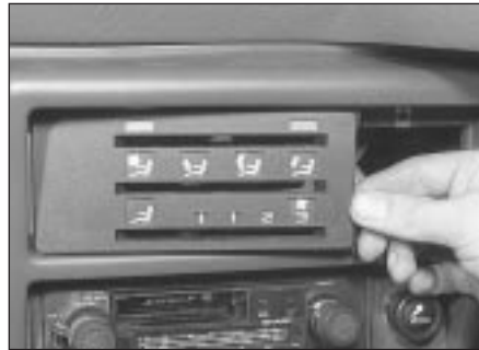
11.8 Heater/ventilation control plate removal
