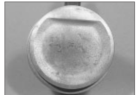
19.16 Arrow mark on piston crowns must point to camshaft sprocket end (letter and number indicate liner and gudgeon pin grade)
