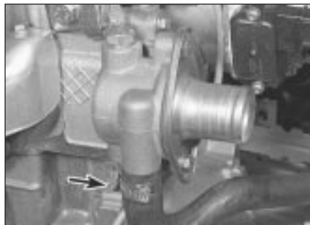
7.8 Water pump hose (arrowed) at thermostat housing
