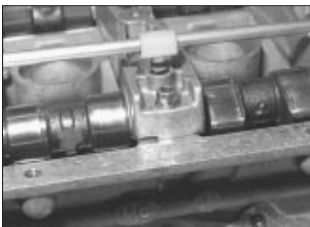
6.33 Camshaft lubrication pipe - note seal on spigot
