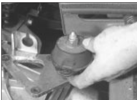
8.30b Removing left-hand engine mounting bracket
