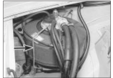
29.3 Spring back the hydraulic reservoir cover retaining clip (arrowed) to release the cover and central block
