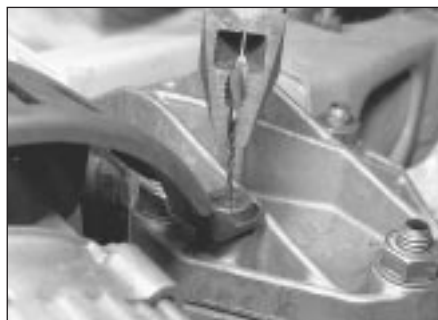
21.8 Method devised for securing alternator guard retaining grommet
