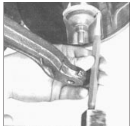
15.8c Carefully drive protector plate into position
