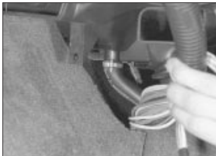
11.27 Heater coolant drain hose
