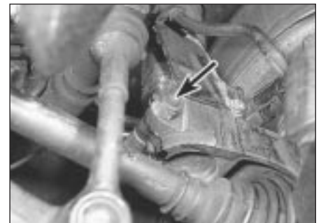
5.8 Swivel hub-to-suspension unit clamp bolt (arrowed)
