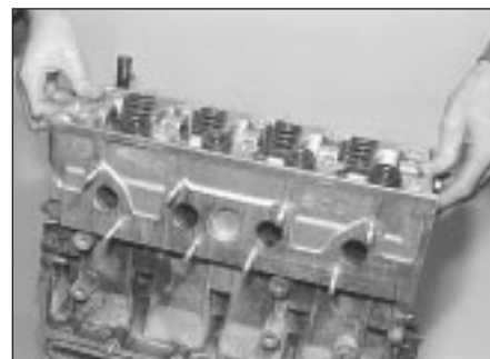
6.34a Lower cylinder head into position . . .
